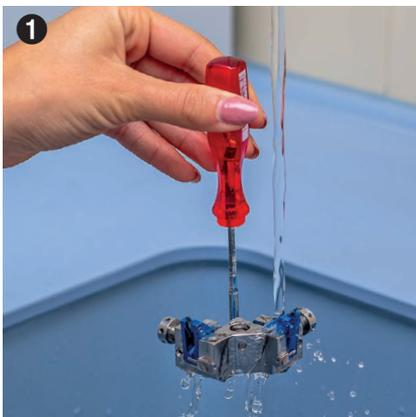
1 Remove the knife stage from the cryo chamber, leave the knives in the stage, wash under tap water for warming up.
