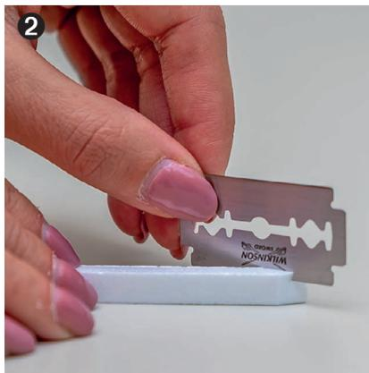
2 Bevel a polystyrene stick with a perfectly clean razor blade.
