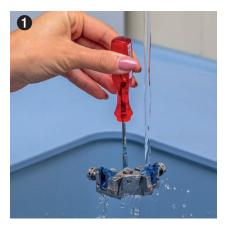
Remove the knife stage from the cryo chamber, leave the knives in the stage, wash under tap water for warming up.
